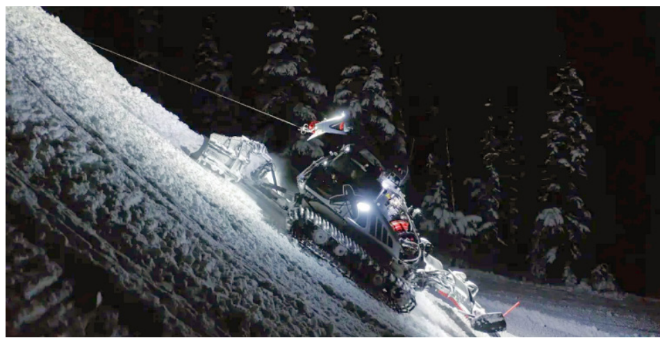
One of the two new snow cats, a Prinoth Bison equipped with a winch, is seen in action grooming a steep slope to provide a smooth, pristine corduroy surface for the skiers and riders soon to come.
