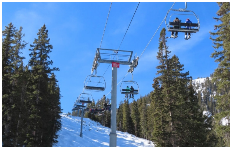
The new fixed grip quad Koala chair comes from the Taos Ski Resort and is shown above from its previous location in New Mexico. It moves 2,400 people per hour up the slope.
