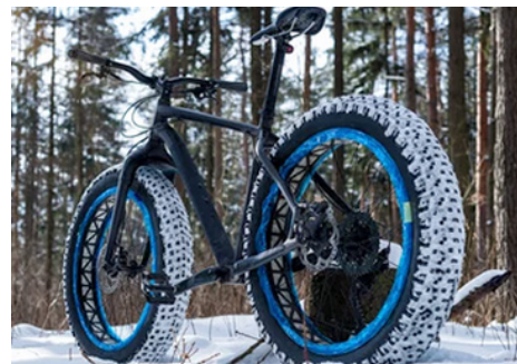
Fat bikes feature tires ranging from 3.5 to 4.8 inches, opening the winter to cyclists.
